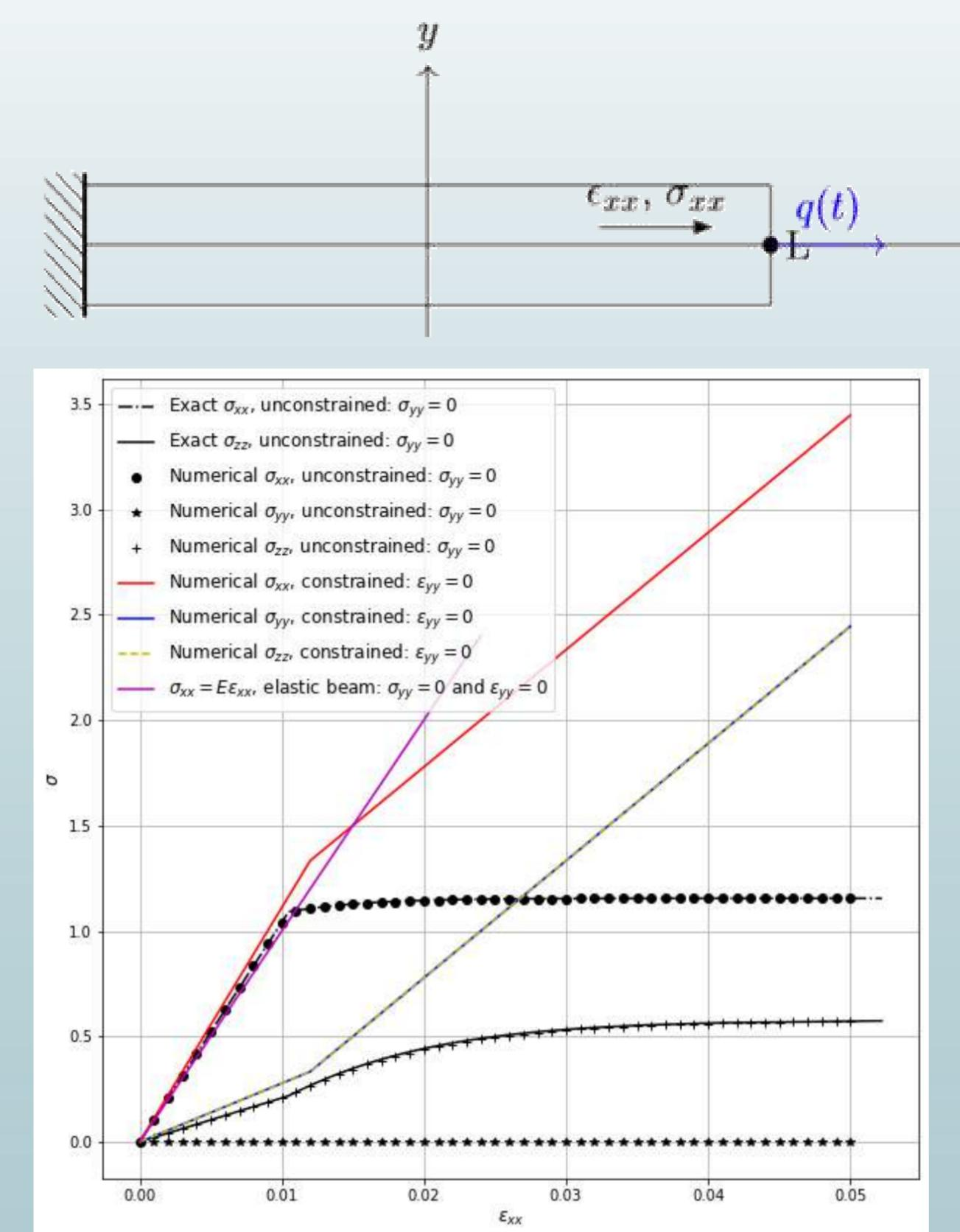
Figure: Stress-strain curves for a 2D elastoplastic traction test [M.Bonnet, 2005], with different modeling assumptions
