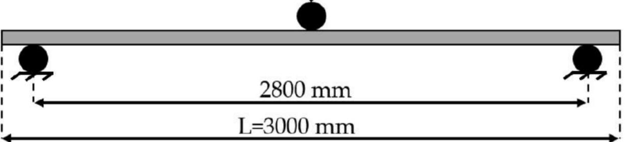
Mechanical diagram of the 3-point bending test
