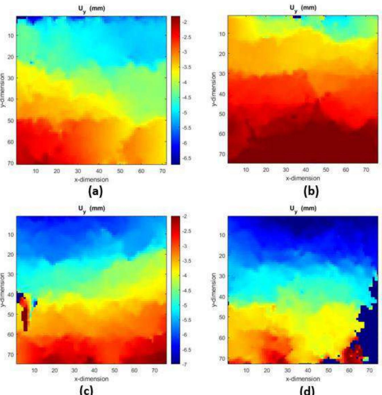
Maps taken at 5.24% of strain, (a): hemp concrete, (b): rapeseed concrete, (c): reed concrete, (d): bamboo concrete
