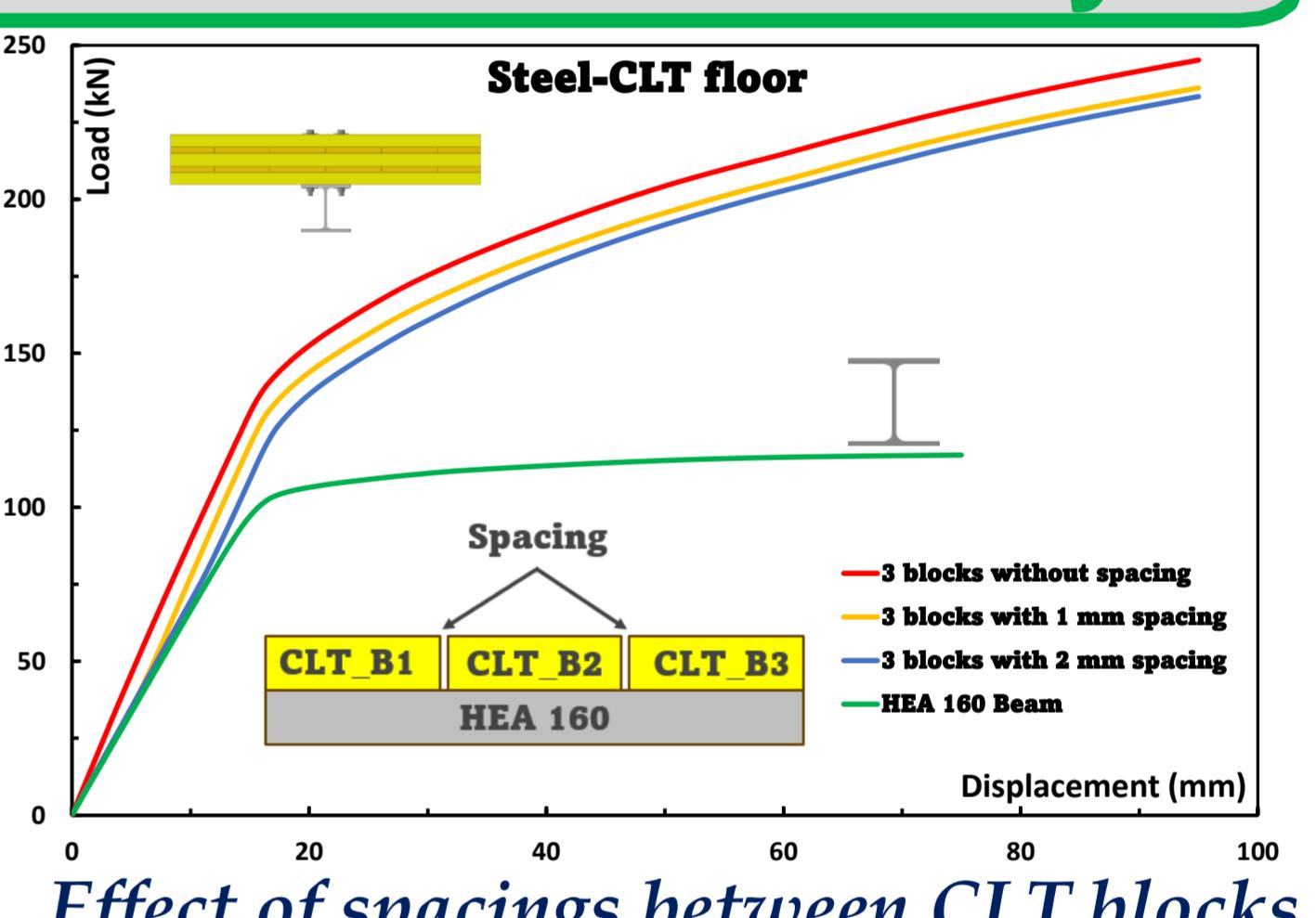
Effect of spacings between CLT blocks
