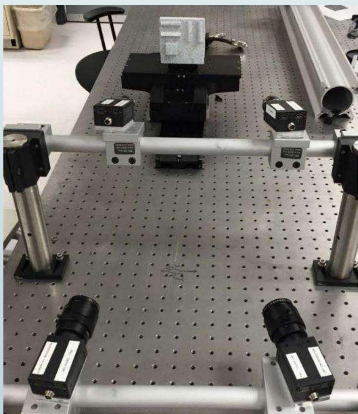
**Figure 1.** Aerotech stage setup with two usual stereo-based camera systems. The front system relies on two 16-mm lenses, and the back system on two 35-mm lenses. (Stereo-DIC Challenge data set [1]).
