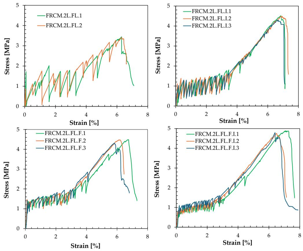
Figure 2. Mechanical behaviour of Flax-FRCM
