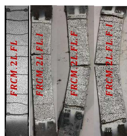
Figure 5. Failure mode of Flax-FRCM
