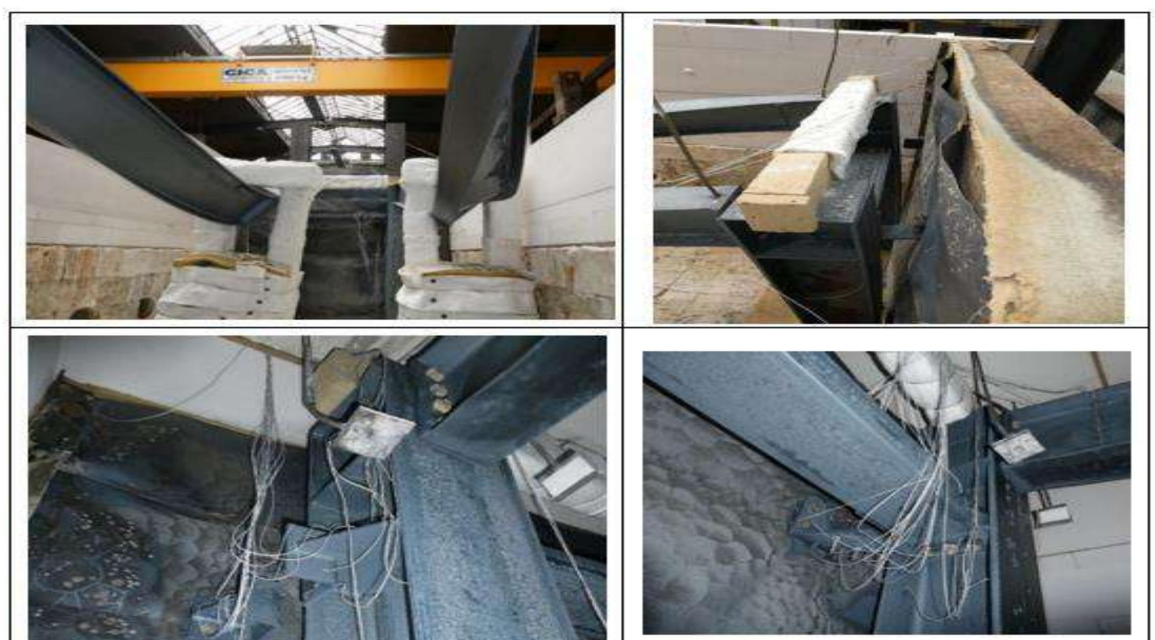
Fusible links after the fire test
