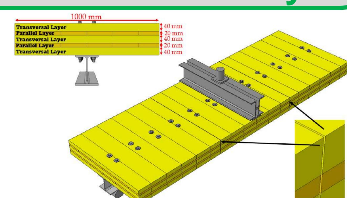
Numerical model of steel-CLT composite floor
