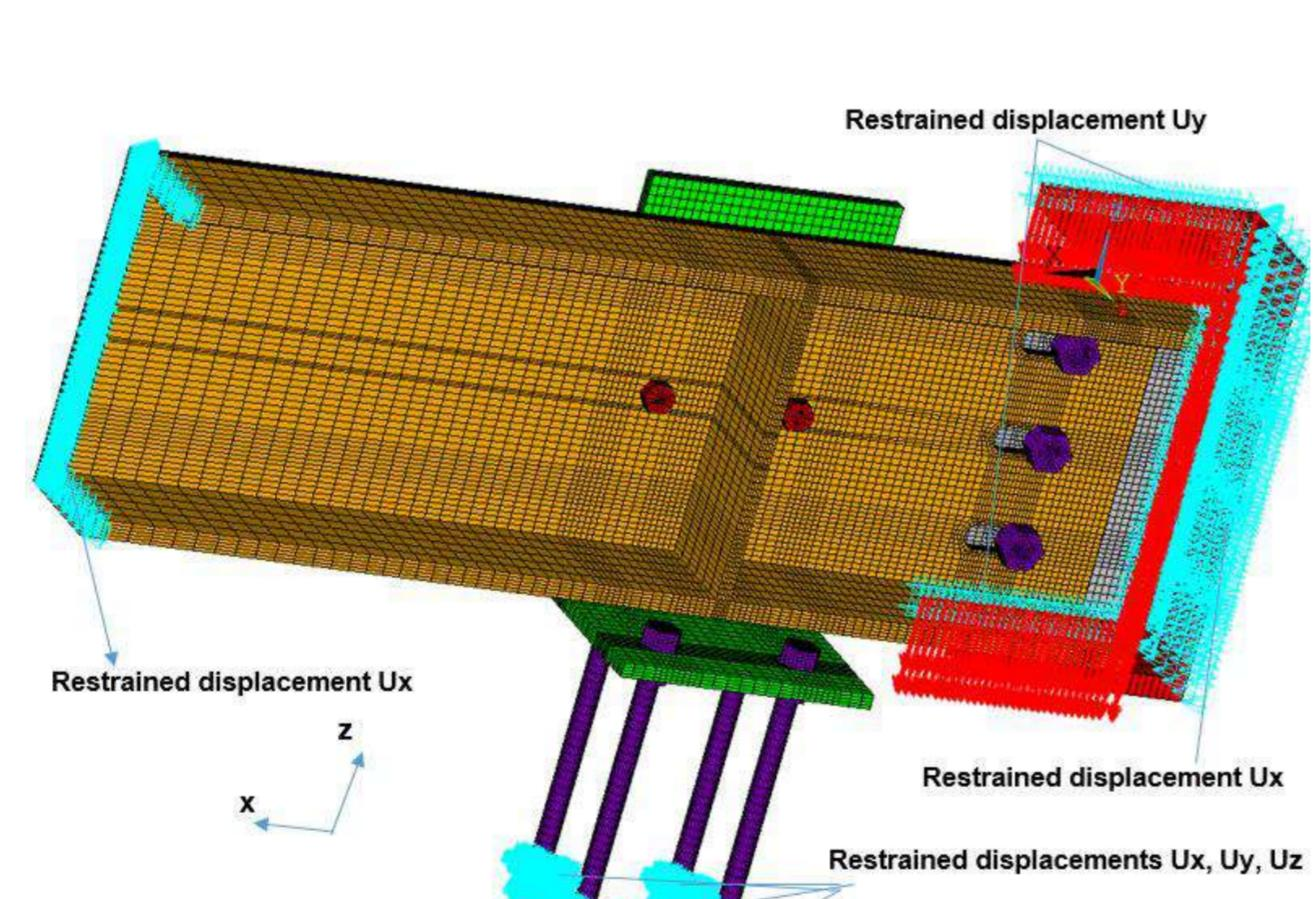
3D FE models for the **mechanical analyses** of fusible links
