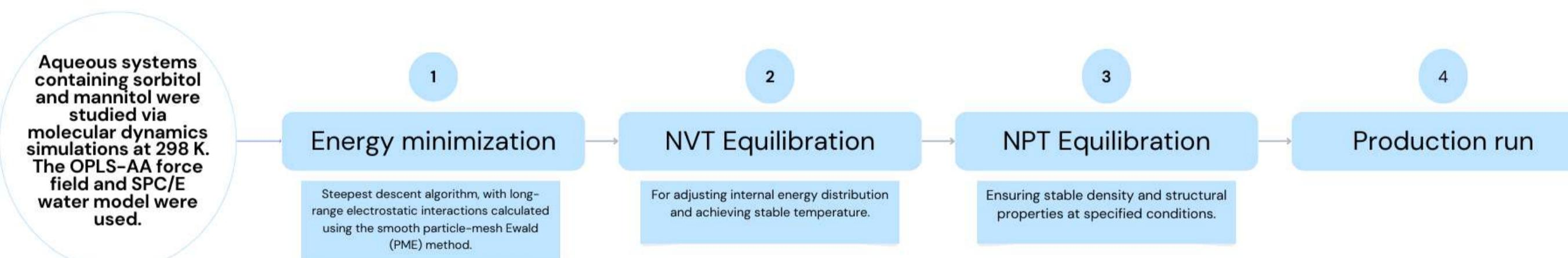
Figure 3: Flowchart of the calculation method on molecular dynamics.
