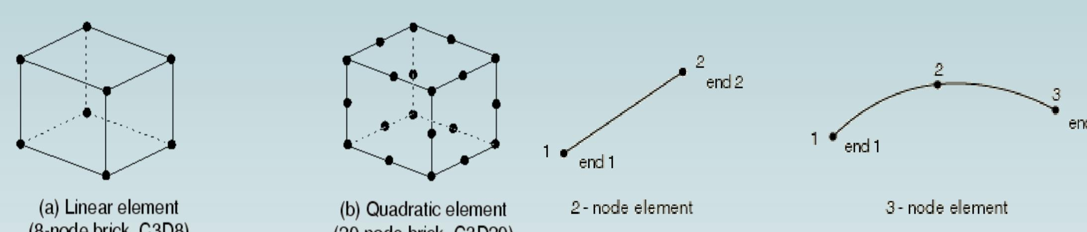
Figure: Continuum solid elements vs beam elements in ABAQUS software
