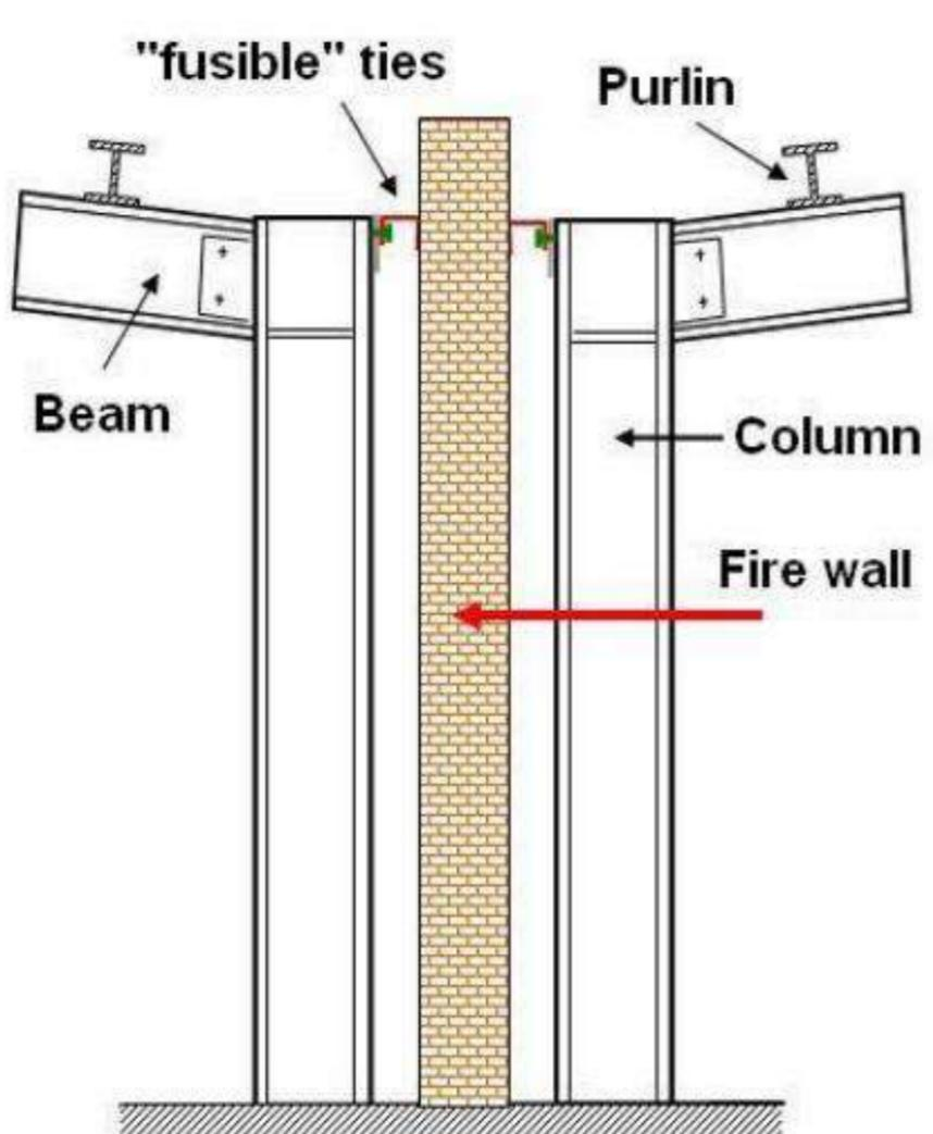
The thesis aims to **study the fire behavior** of "fusible" links for fire-walls installed in single-story steel buildings using :
