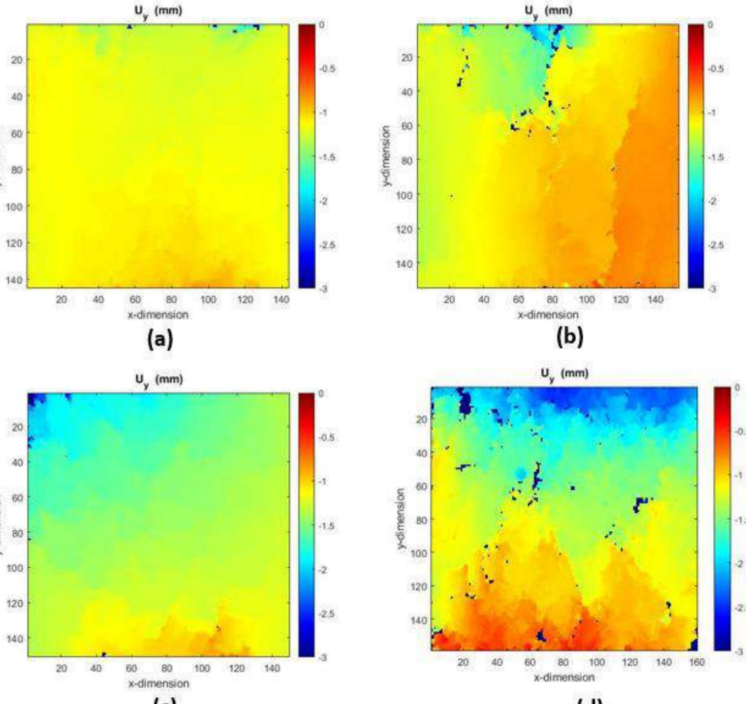
Maps taken at 2 % of strain, (a): hemp concrete, (b): rapeseed concrete, (c): reed concrete, (d): bamboo concrete
