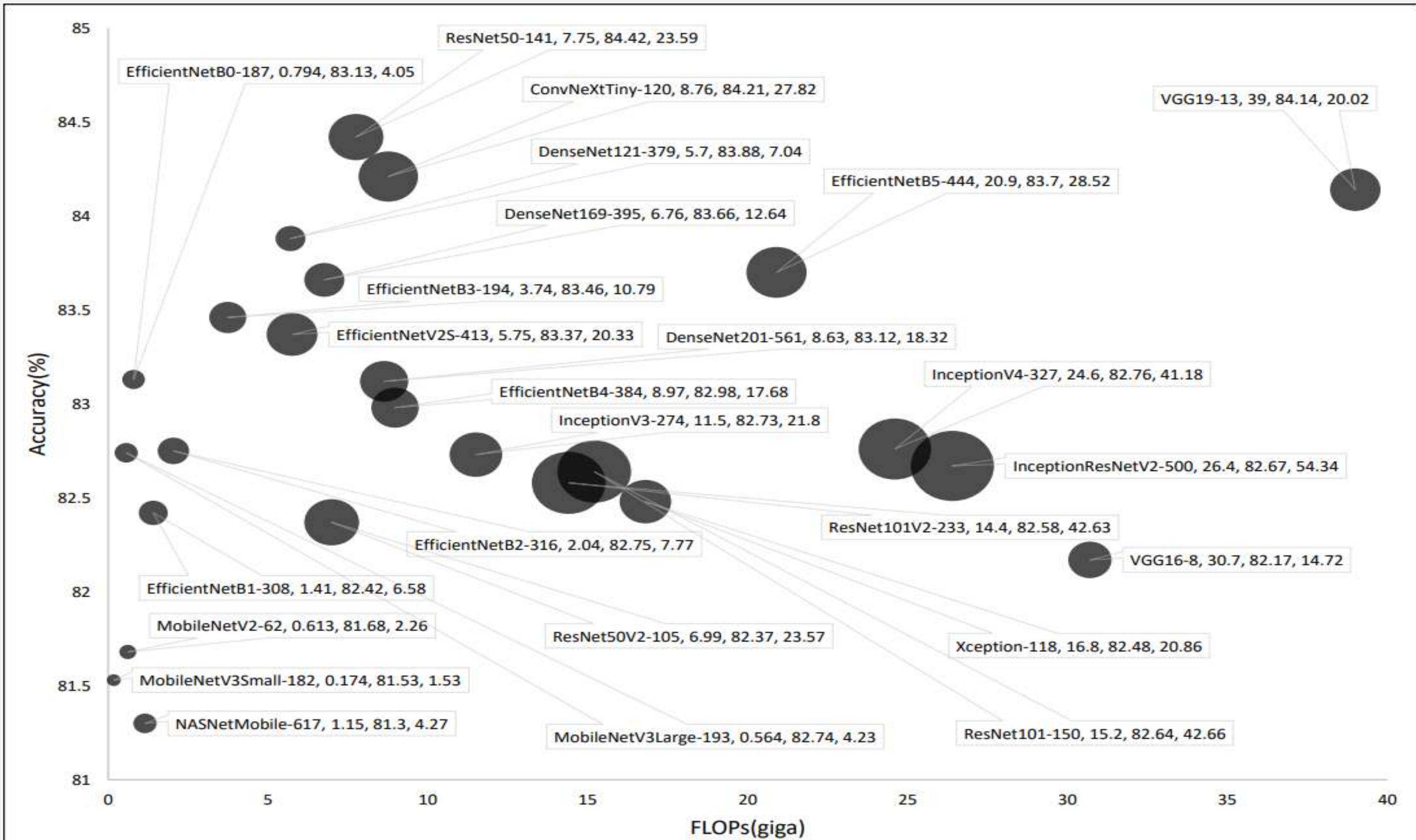
Model accuracy vs floating point operations. Bubble size represents the number of parameters.
