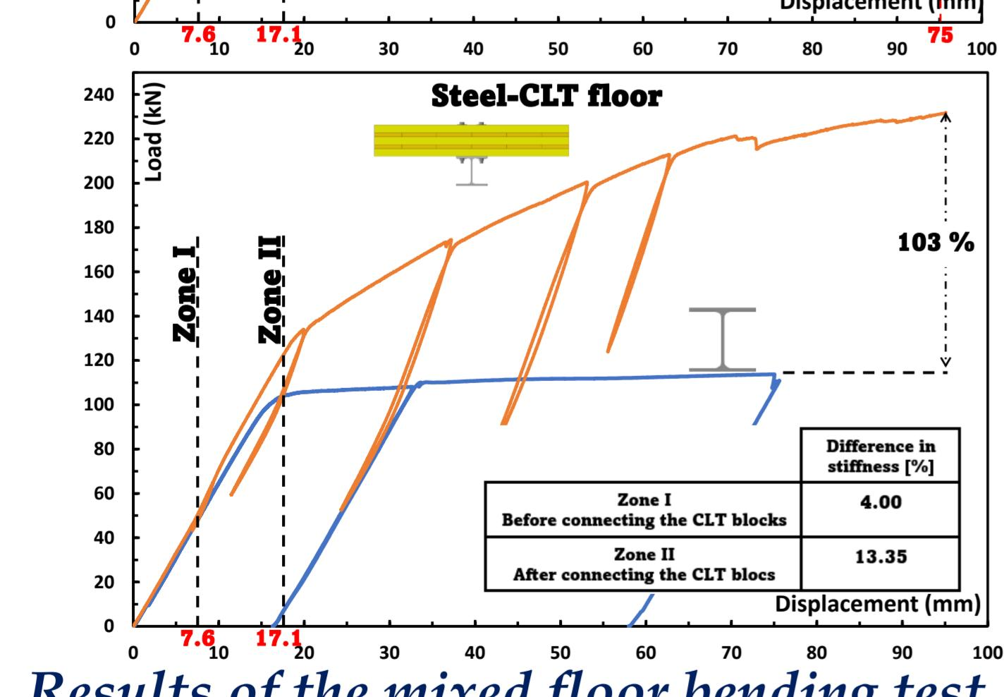
Results of the mixed floor bending test
