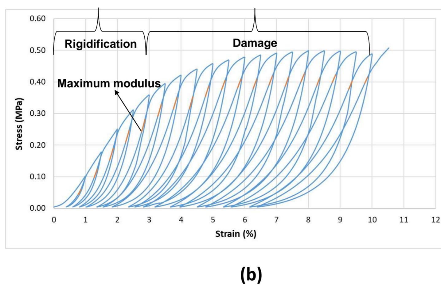
Example of cyclic compression stress-strain curves for a particular bio-based specimen (CEMIV-Hemp) with 19 cycles of loading-unloading, and the exploitation methodology of the floating modulus (orange lines) for the two aggregates' orientation, (a): parallel orientation ; (b): perpendicular orientation.
