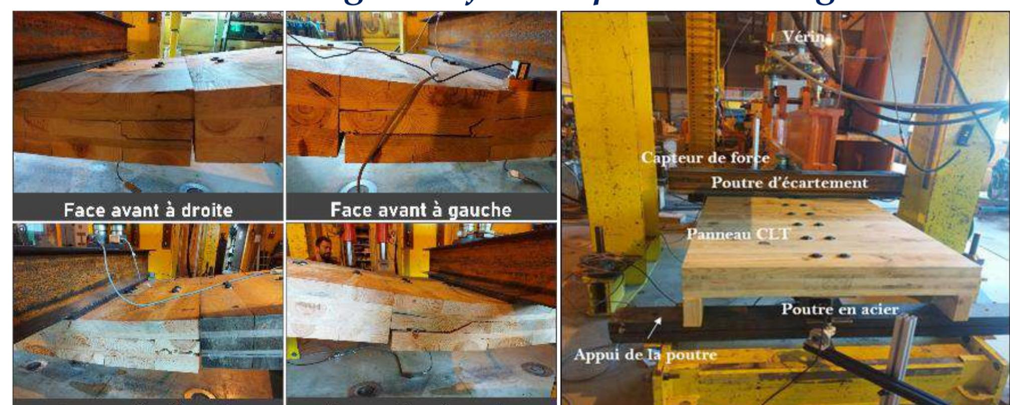
Three-point bending test of the composite floor
