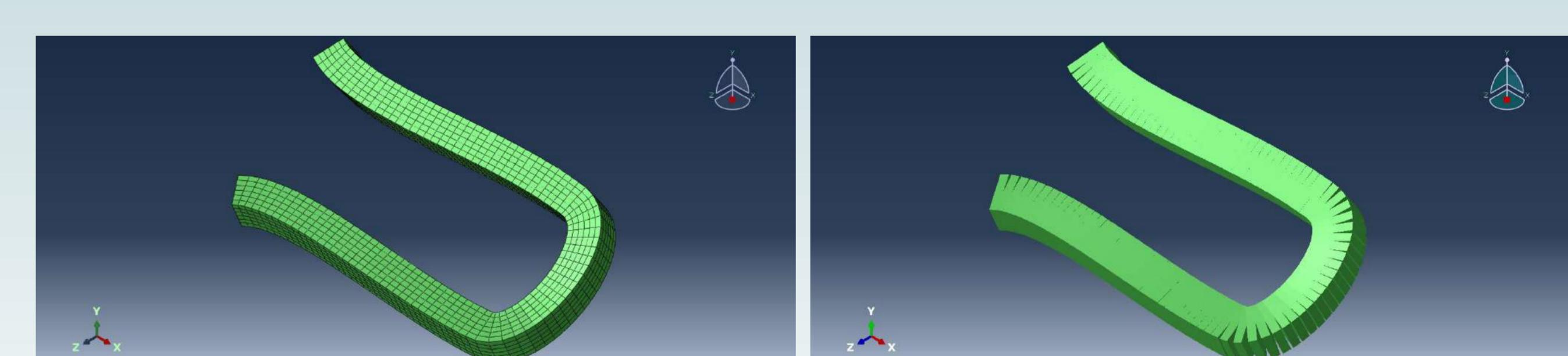
Figure: Stent (Ultimaster Nagomi by Terumo) modeling and inflation in ABAQUS
