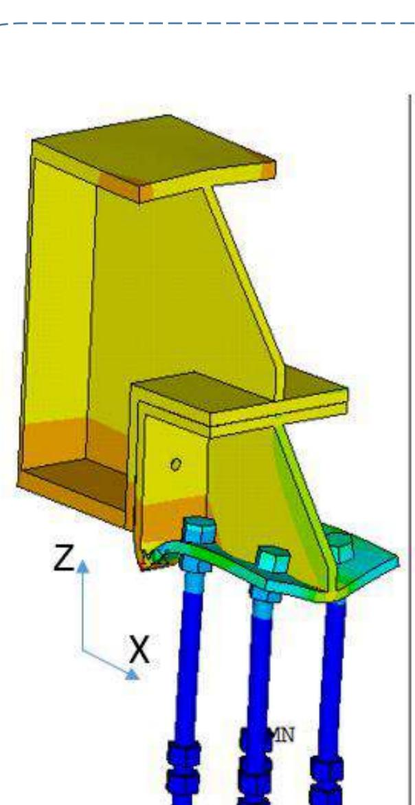
Deformed shapes of fusible links at failure time
