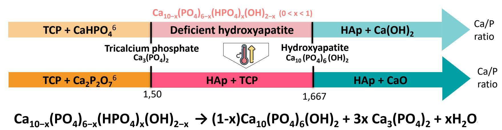
BCP has been synthesized through the co-precipitation of deficient HAp, followed by a thermal treatment allowing HAp and TCP formation. In the HAp structure, **strontium** ions replace calcium ions, preferentially on less dense Ca(2) site (Wyckoff 6h), and **zinc** and **copper** ions are inserted and thus form an interstitial solid solution at the Wyckoff 2b sites.<sup>6</sup>
