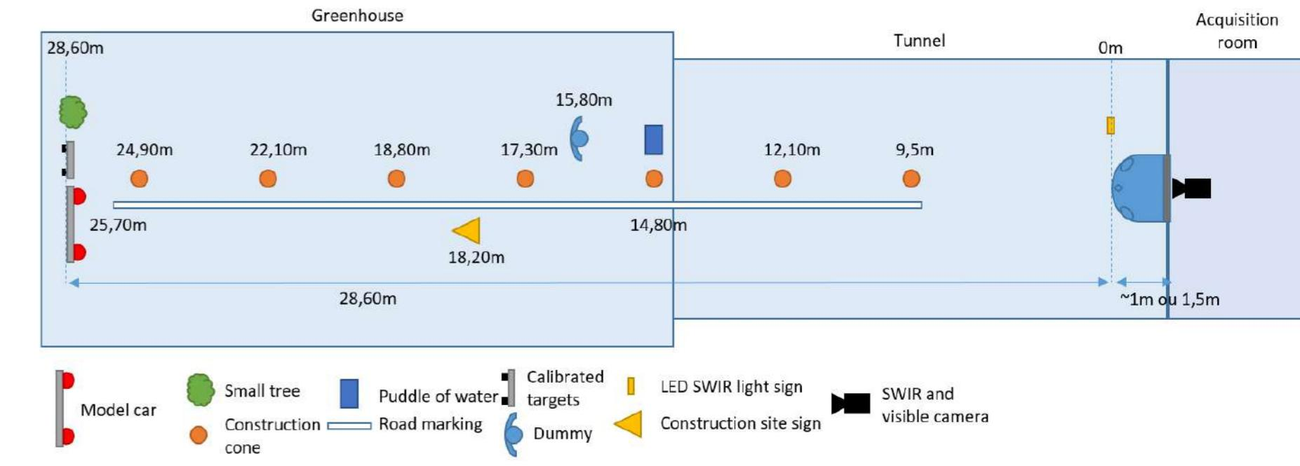
Figure 3: Diagram of the acquisition process at Cerema.
