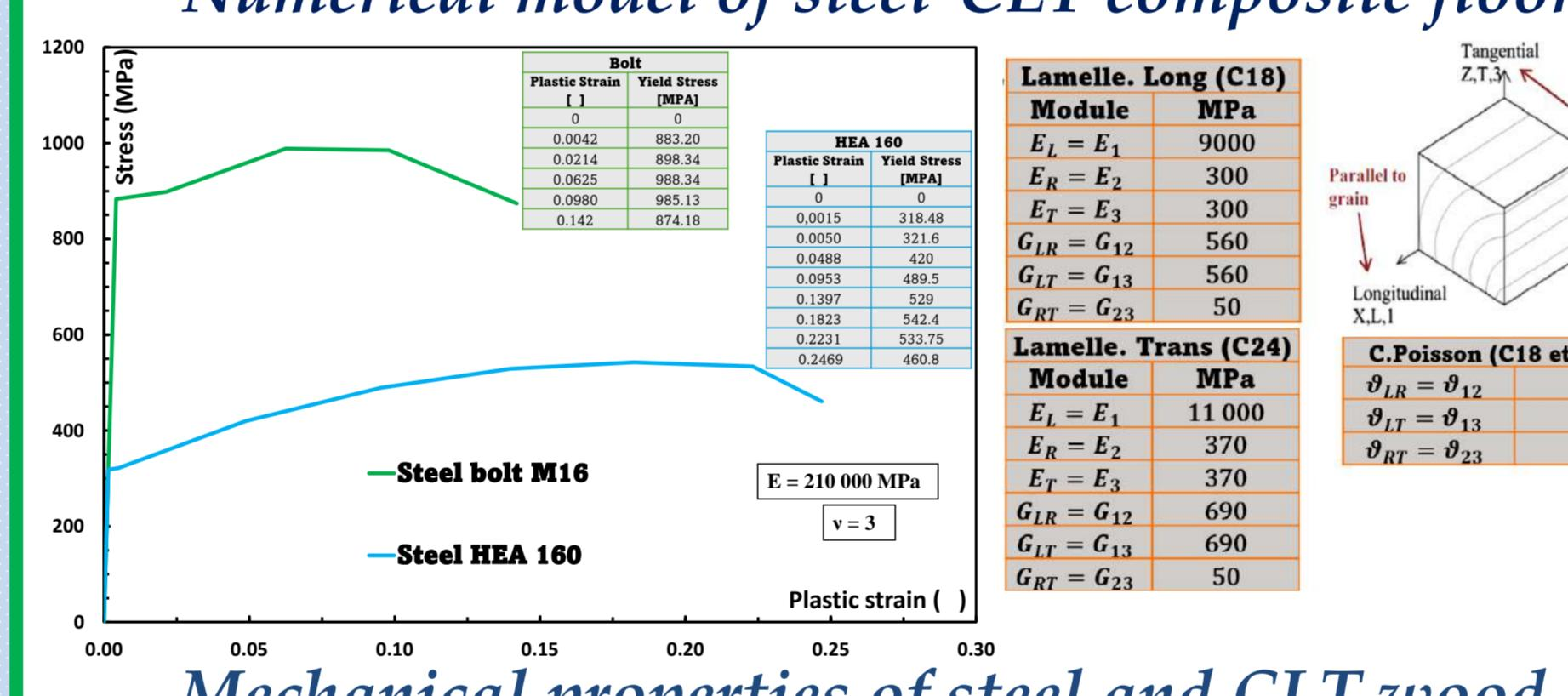
Mechanical properties of steel and CLT wood
