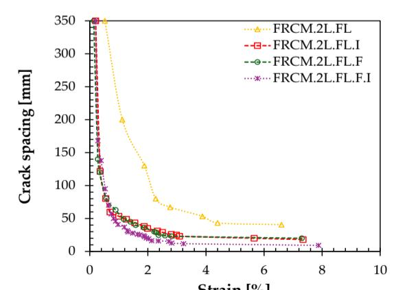
Figure 4. Crack spacing evolution of Flax-FRCM
