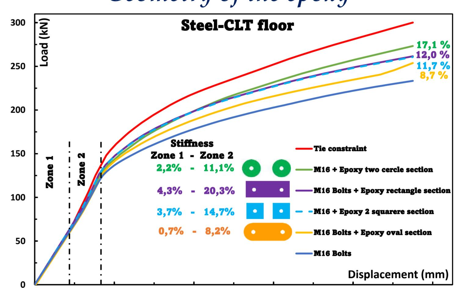
The effect of epoxy presence on the mechanical behaviors of composite floors
