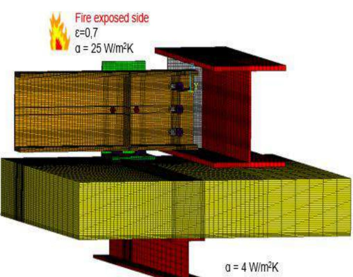
3D FE models for **thermal analyses** of two fusible links
