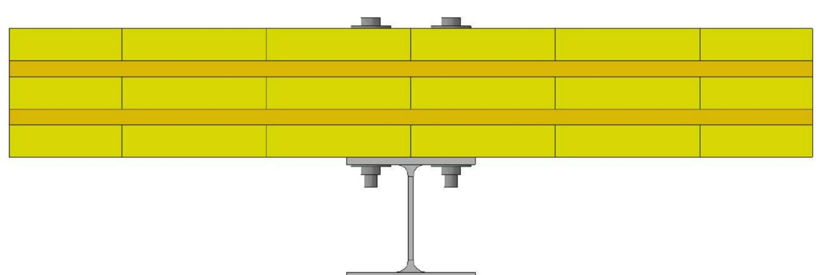
Cross-sectional view of steel-CLT composite floors
