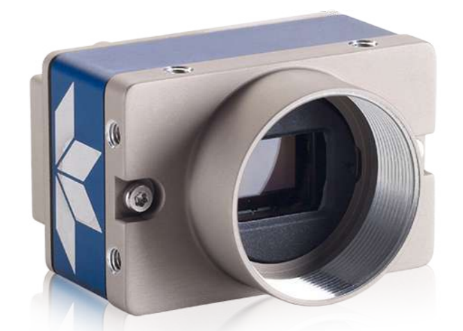
Figure 10: Genie Nano C1630 RGB Camera
