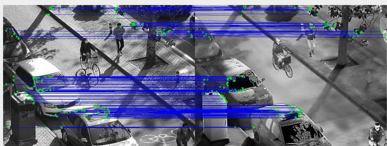
Fig. 7: Matched keypoints between thermal and visible.
