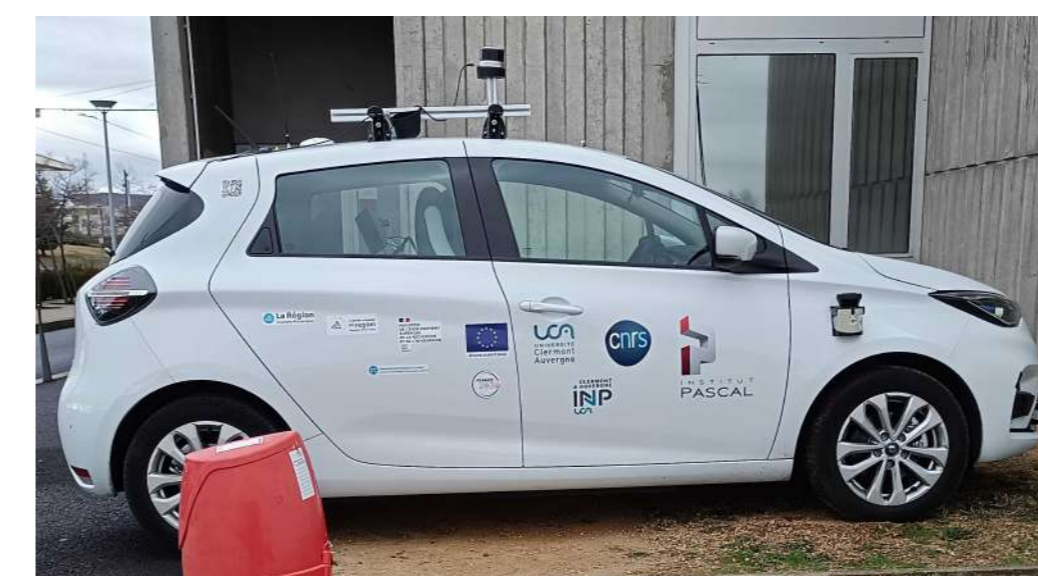
Figure 11: Renault Zoé modified for autonomous driving
