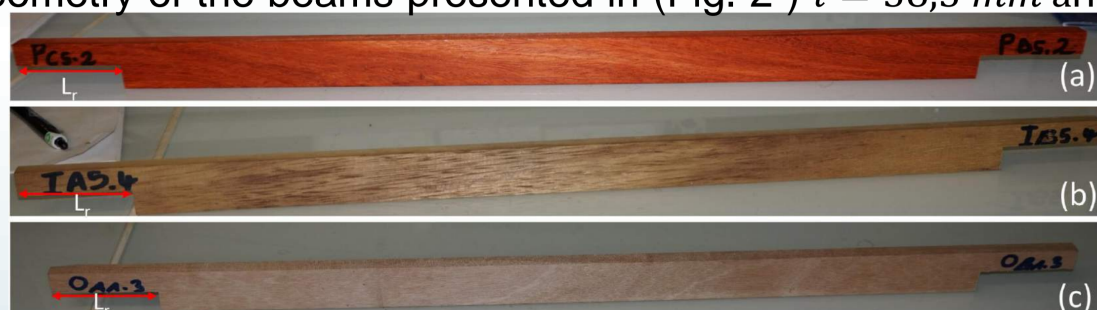
Fig 2. Geometry of test specimens (a); Padouk (b) Iroko (c); okume
