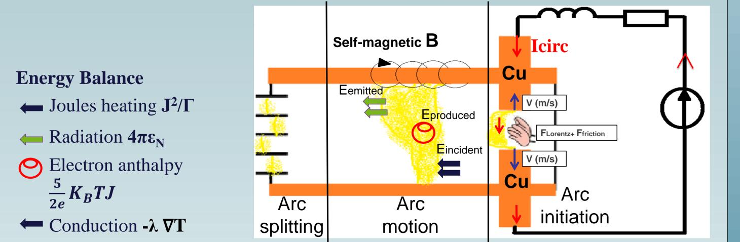
The air arc in switches typically exists near atmospheric pressure; its temperature is usually of the order of 10 kK. So as initial condition a rectangle surface between the moving contacts with 10kK temperature is taken (T=0s). The results show the arc elongation with the moving contacts after 0,05 ms, and its propagation in the chamber to the splitter plates during the time.
