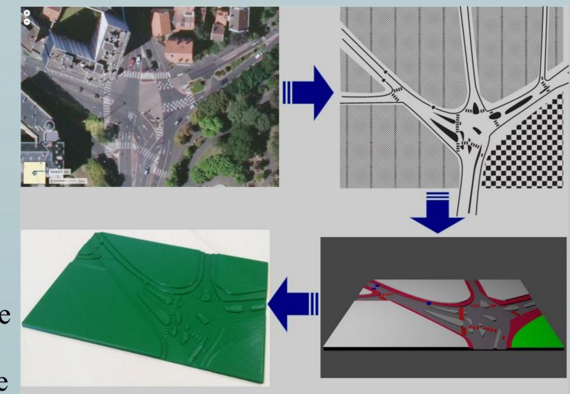
Top left Aerial view (© IGN, Geoportail), top righ adapted image by MARTIN Durga (© CRDV), bottom left 3D model and bottom right the printed model made by ourselves
