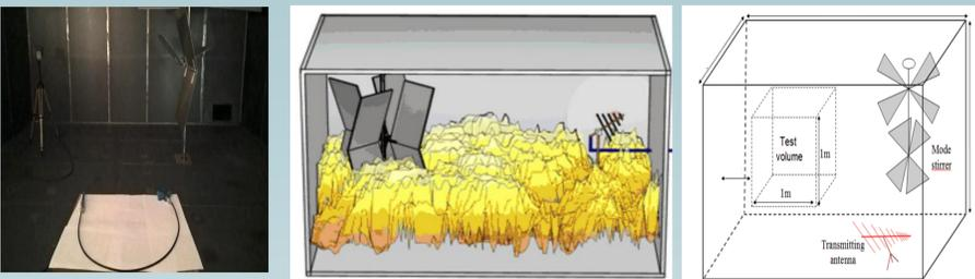
It should be noted that for the cable transfer impedance measurement benches previously mentioned, the shielding is subjected to a TEM wave. Screening effectiveness measurements of RG58 type cable samples will be carried out using several methods and the results obtained will be validated by comparison with theoretical data (obtained from transmission line theory and MS CST).
